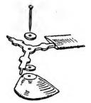
Fig. 2.—Details of the rotor hub arranged in order of assembly.
